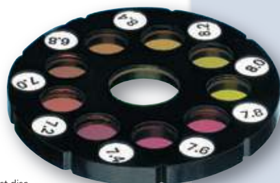
Test disc with colour stable glass standards
